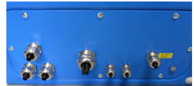
Threaded fitting M16 for power supply
