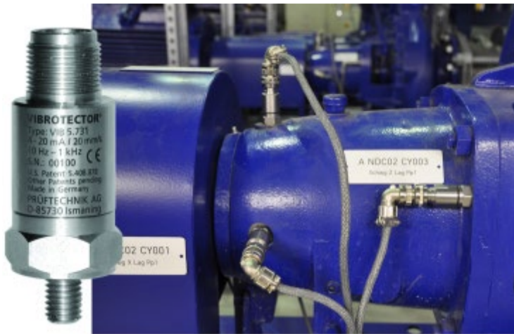
Monitoring vibrations with VIBROTECTOR
